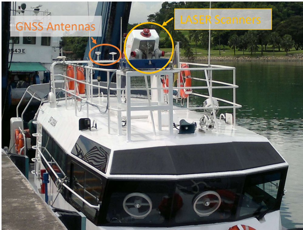
Simultaneous survey with Multibeam and LASER Scanner System
